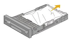
3 Pull the jammed paper out carefully to avoid tearing it. If you are still unable to remove the paper, go to the next step to remove the jammed paper from the inside of the printer.
